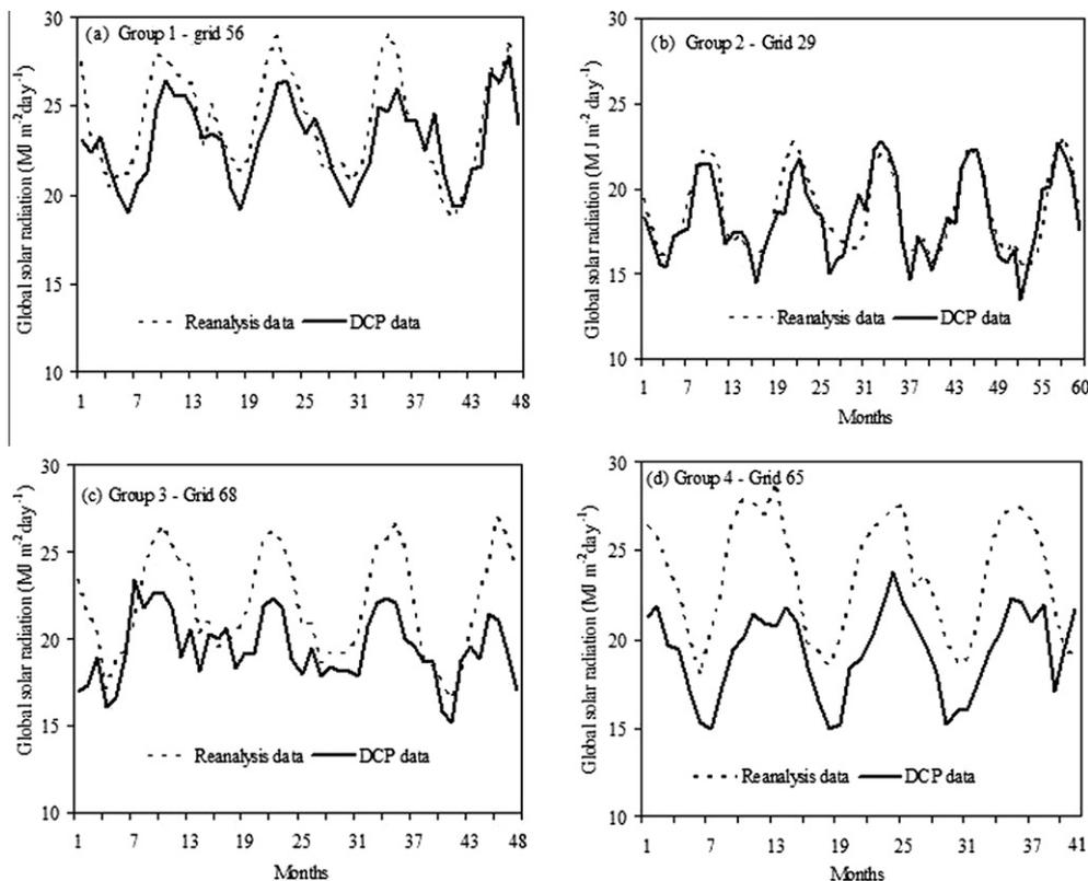
Fig. 5. Comparison of monthly global solar radiation (MJ m<sup>-2</sup> day<sup>-1</sup>) from re-analysis and measurements by data collection platform (DCP) for four select grid points in northeastern Brazil.
