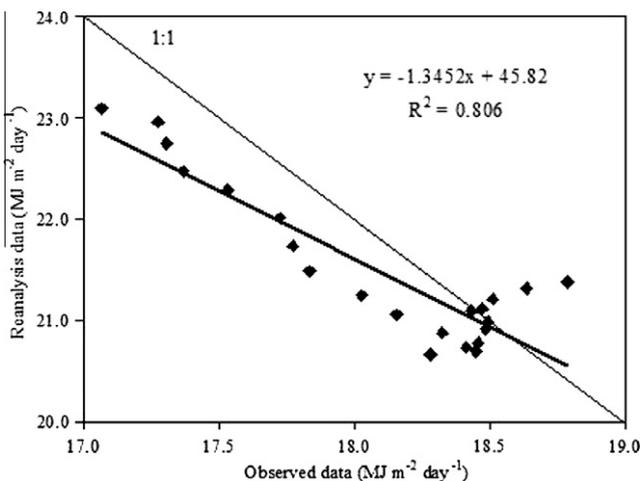
Fig. 6. Relationship between re-analysis and measurements data at grid point 46 (mean values for Petrolina and Juazeiro stations) of global solar radiation ( $\text{MJ m}^{-2} \text{ day}^{-1}$ ).
